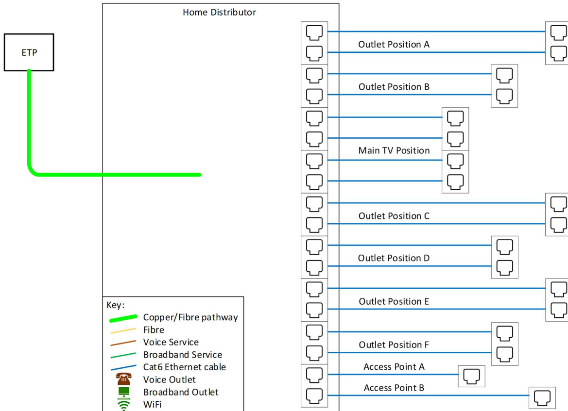
Figure 8: Generic Cabling System Components
